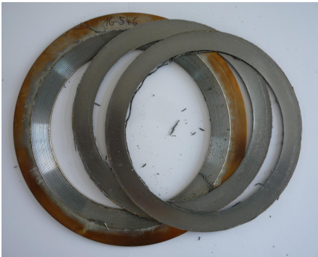
Fire test according to API 6FB (MESC SPE 85/300 - 3.3.3)
